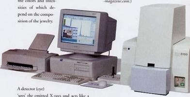
'sees' the emitted X-rays and acts like a prism to separate them into the different colors, or wavelengths, and convert them into distinct electronic signals. The signals are sent through the electronics to the computer (brain), where they are processed into elemental composition as a percentage of gold, silver, copper, etc. The main difference is that XRF is using 'colors' that are invisible to us, but not to the instrument.
